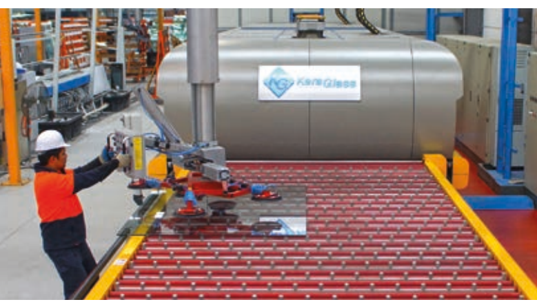
◀ Toughening furnace, Smithfield
