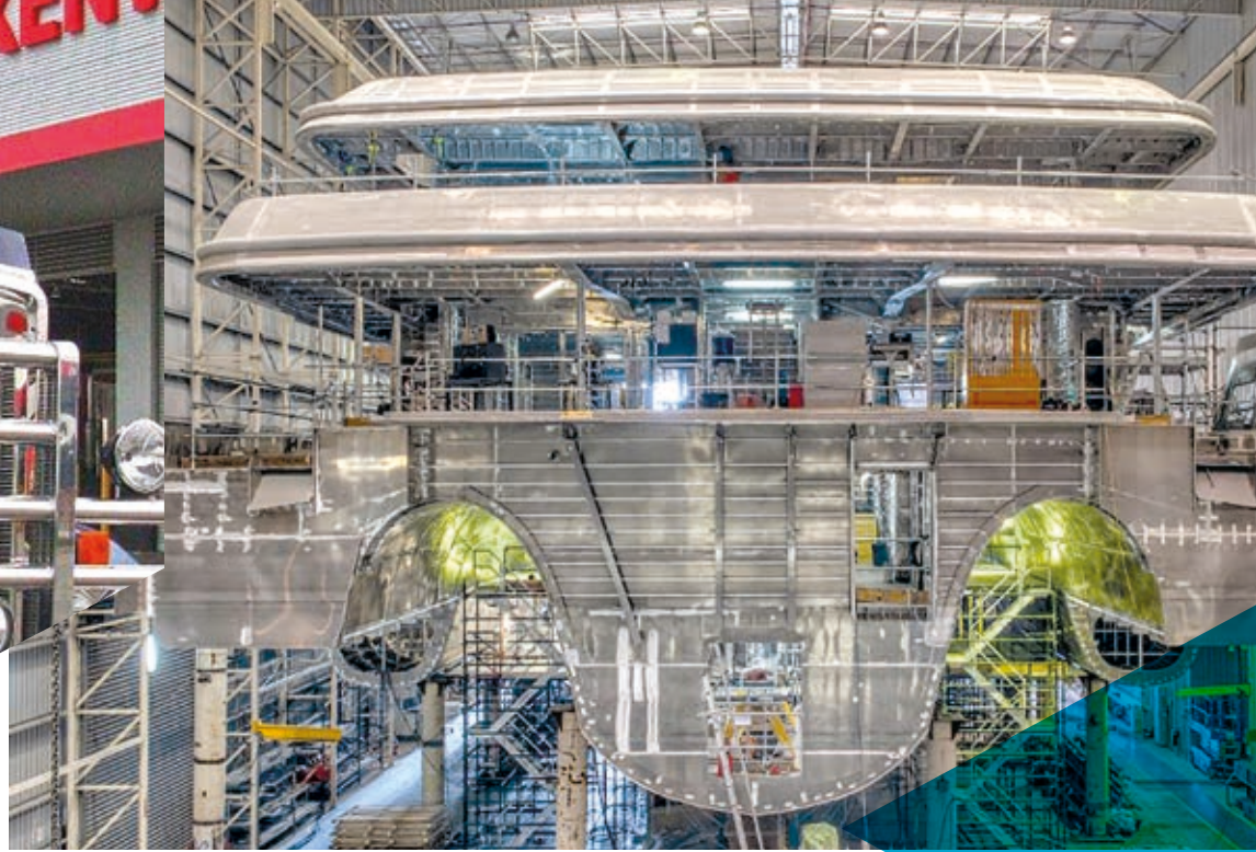
▲ G.James supplied marine certified aluminium sheet, plate & extrusions to Echo Yachts – 84m luxury trimaran project. (Photo courtesy of True North Mark)
