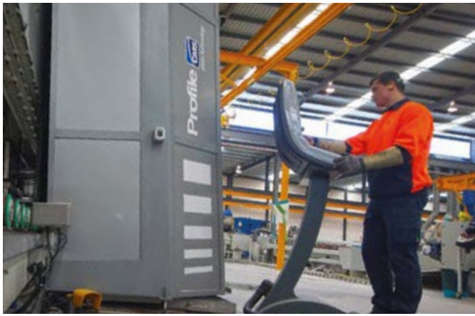
▲ Programming vertical CNC machining centre
