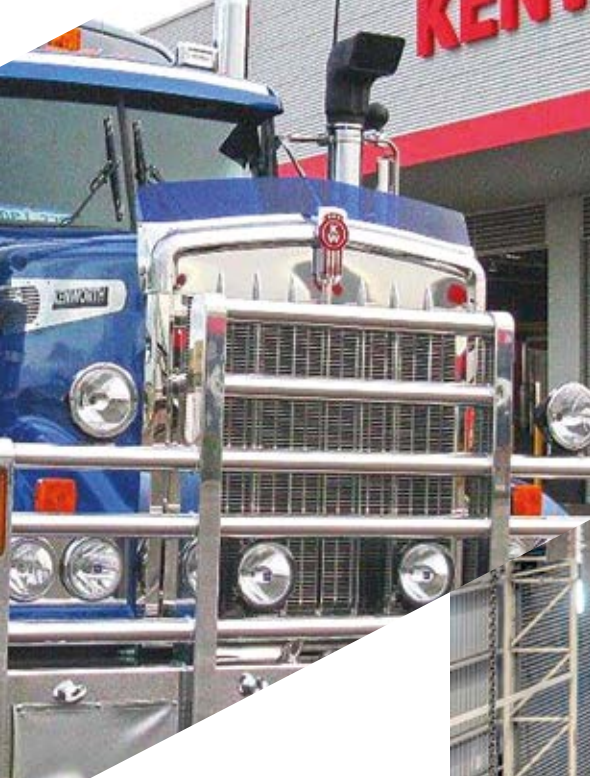
▲ Extruded aluminium profiles supplied for the manufacture of heavy vehicle bullbars. (Photo courtesy of K-Craft)
