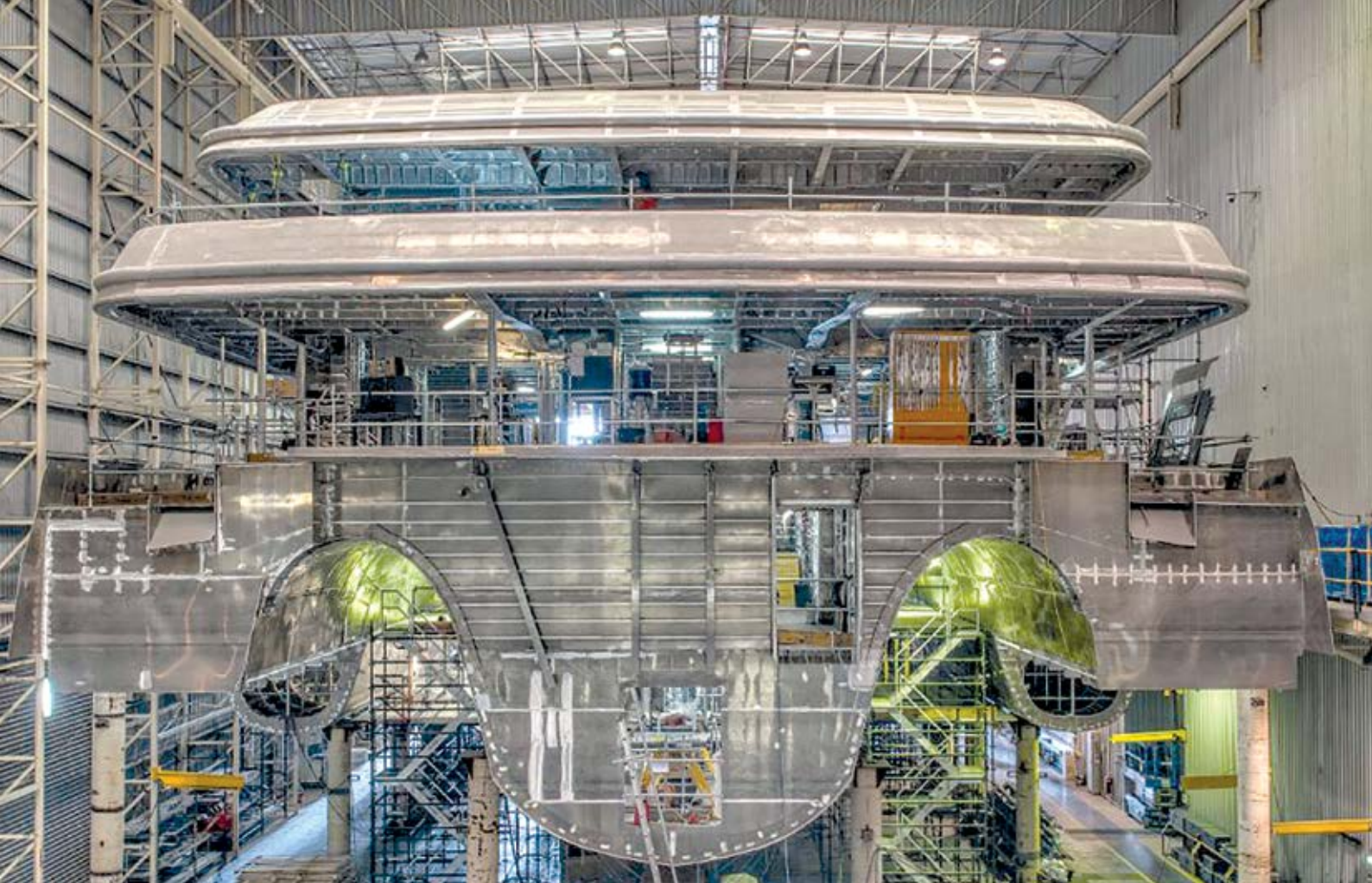
White Rabbit Golf: the largest superyacht built in Australia and the largest aluminium, tri-hull superyacht in the world at 84 meters and nearly 3000 gross tonnes.
