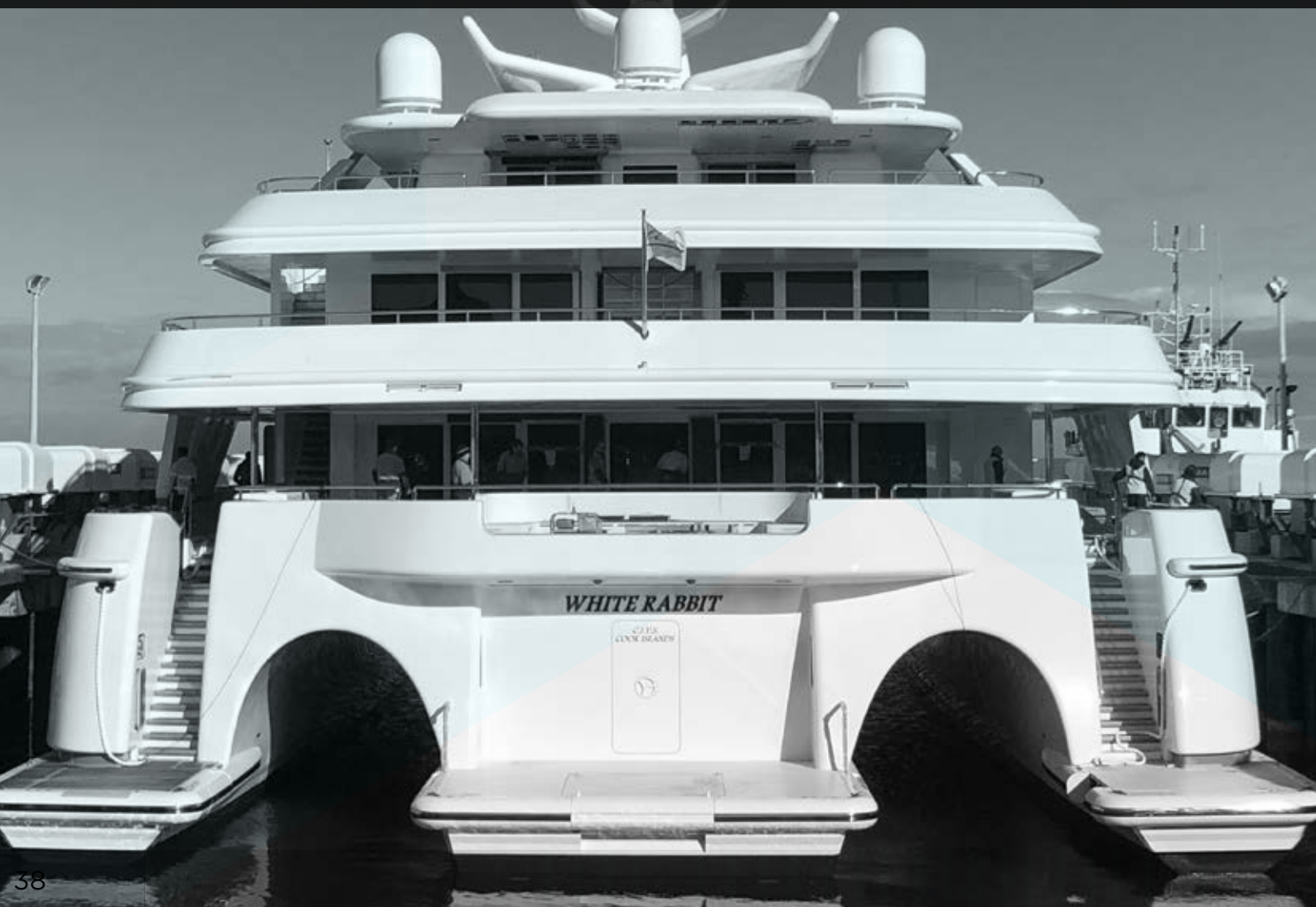
White Rabbit Golf: the largest superyacht built in Australia and the largest aluminium, tri-hull superyacht in the world at 84 meters and nearly 3000 gross tonnes.
