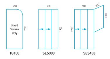
(Toughened glass panel only, aluminium framing to wall & floor)
